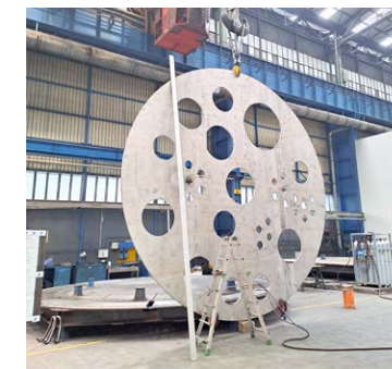
Figure 3: First portion of the SPARC cryostat base weldment. The various holes are for connections to systems within the cryostat including electrical and cooling for the superconducting magnets.
