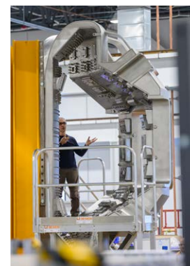
Figure 1: Full-scale 60-degree mockup of SPARC vacuum vessel at the CFS facility used for testing internal components.
