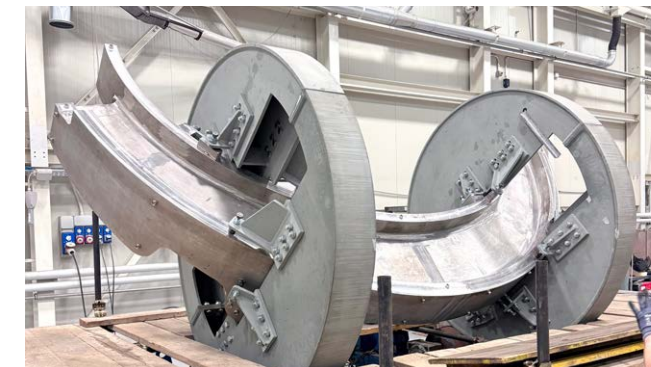
Figure 2: Portions of a toroidal field magnet structural case in a welding fixture.
