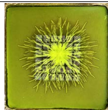
Above: Schematic illustration of a cross-section for air discharge to touchscreen surface. Right: Example of dust figure on touchscreen surface
