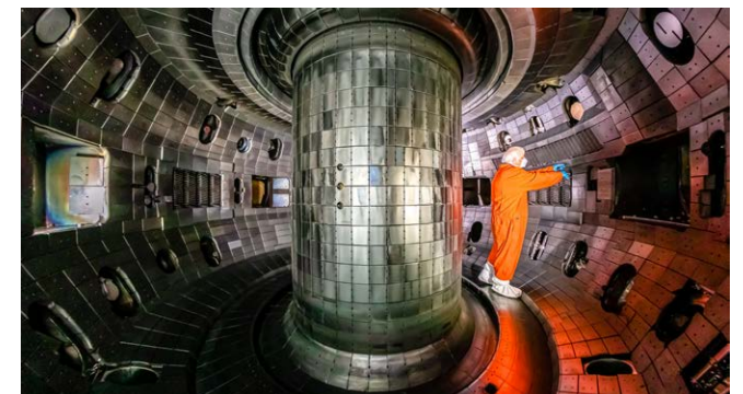
Figure 1b. Internal view of the tokamak at the DIII-D National Fusion Facility in San Diego.
