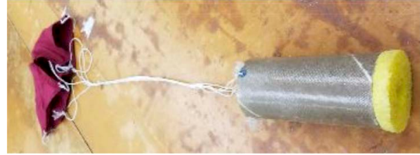
Fig. 10. Air-delivery capsule with attached drogue chute
