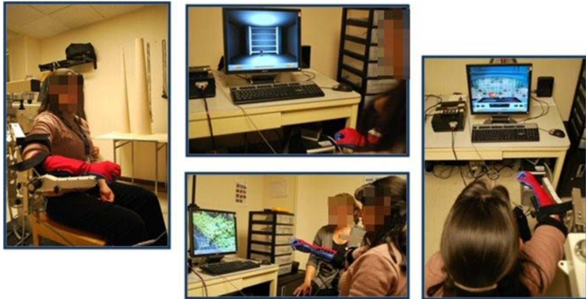
Fig. 6. Rehabilitation robotics is combined with wearable technology for the purpose of enhancing functions that are not provided by robotic systems [51]. Features provided by commercially available robotic systems like the one shown in this figure (Armeo by Hocoma AG) can be augmented via the use of wearable sensors. In the example presented, a sensorized glove provides the system with the ability to implement exercises targeting the recovery of hand function. This capability would not be available if the robot were to be used alone.
