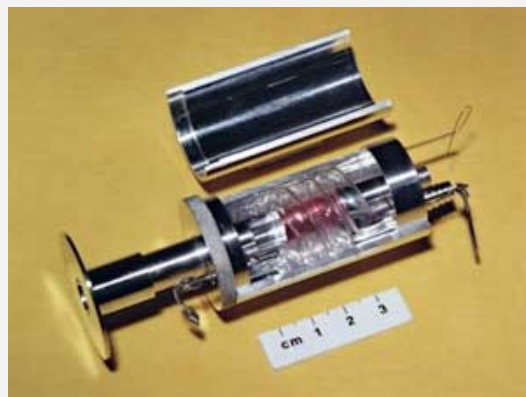
The first successful working laser, constructed by Dr. Ted Maiman in 1960. Courtesy: HRL Laboratories, LLC.
