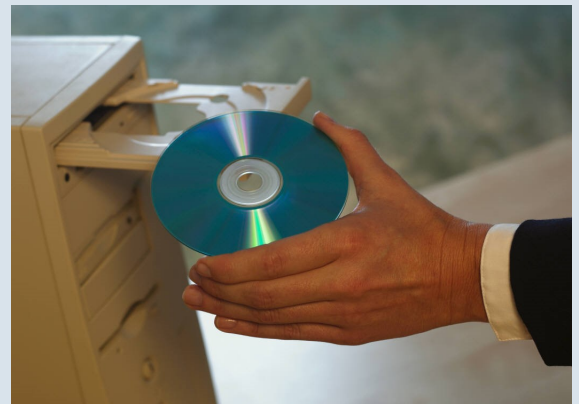
CD-ROM read and write components contain a laser diode that is not safe if viewed directly during operation.
