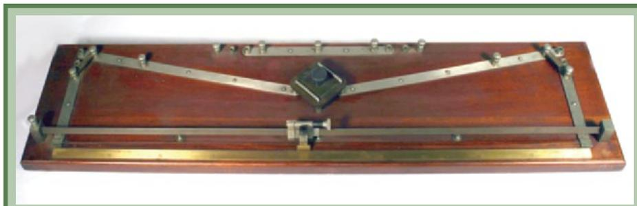
Figure 1. 1903 L&N Wheatstone Reversible Meter Bridge
