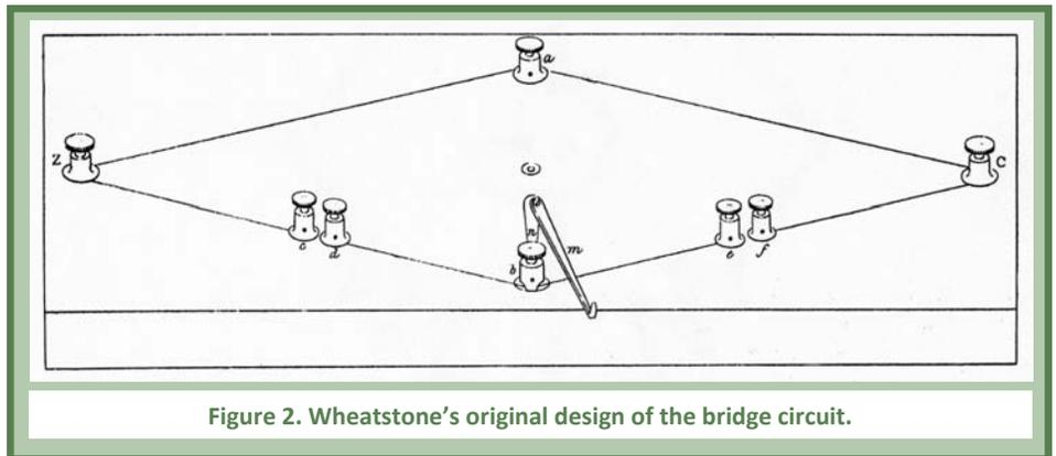
Figure 2. Wheatstone's original design of the bridge circuit.
