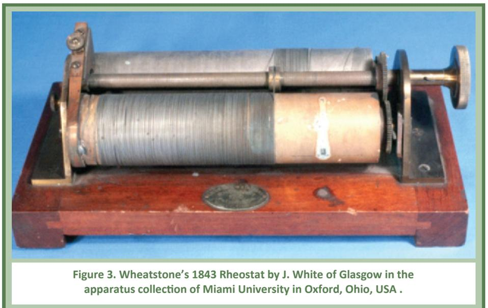
Figure 3. Wheatstone's 1843 Rheostat by J. White of Glasgow in the apparatus collection of Miami University in Oxford, Ohio, USA .
