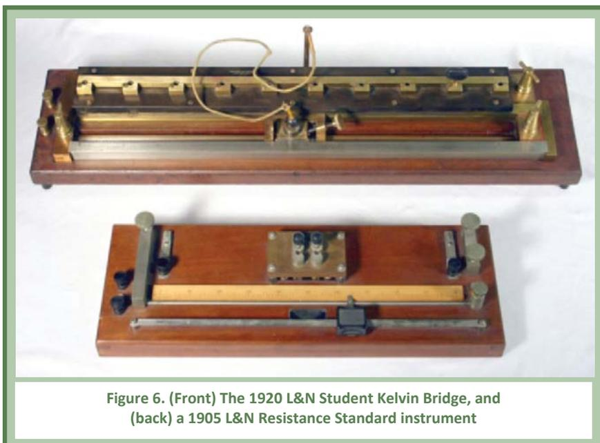
Figure 6. (Front) The 1920 L&N Student Kelvin Bridge, and (back) a 1905 L&N Resistance Standard instrument
