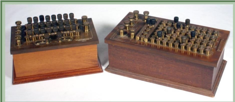
Figure 4. (L) The classic 1903 L&N Post-Office Pattern Wheatstone Bridge, and (R) the 1907 L&N Decade Resistance Box and Wheatstone Bridge.
