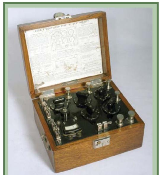
Figure 5. The 1914 L&N Type S portable testing Wheatstone bridge
