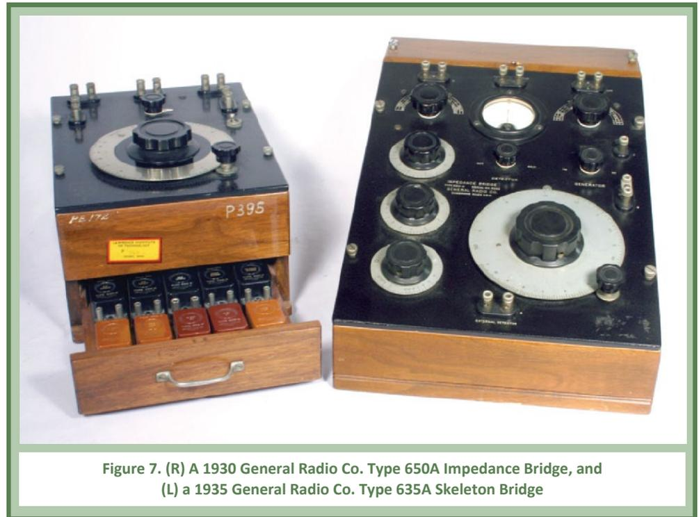
Figure 7. (R) A 1930 General Radio Co. Type 650A Impedance Bridge, and (L) a 1935 General Radio Co. Type 635A Skeleton Bridge
