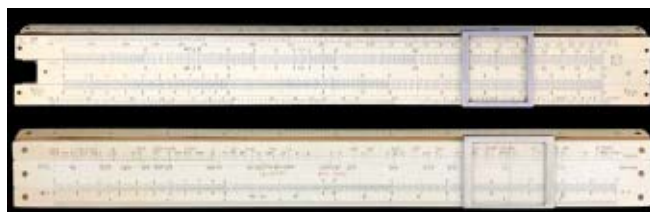
Fig. 6. Top: Model 378 Electro slide rule, 1913, by Faber-Castell, Germany. Bottom: Model 33 Chemical slide rule, 1928, by Nestler, Germany.
