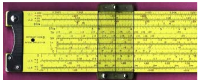
Fig. 22. Pickett Model N4-ES Vector Type Log-Log Duplex Slide Rule with Eight Log-Log Scales
