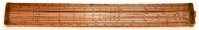
Fig. 8. A Sliding Gunter with Logarithmic Sine and Tangent Scales on both Stator and Slide to Facilitate Calculations Dealing with Navigation
