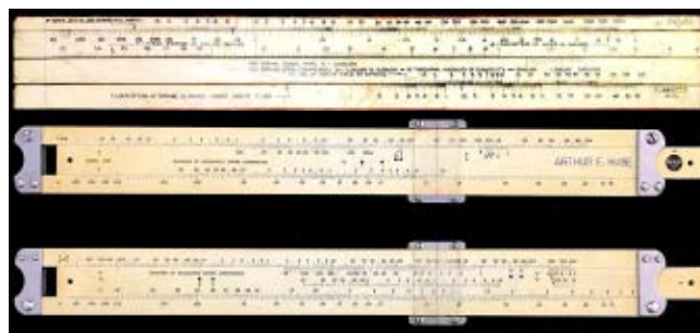
Fig. 7. Spring design slide rules. Top: Rule with 2 slides made by R. K. Baetzmann, 1941, Chicago. Bottom: Model 1025 (front and back), 1952, by Pickett, Chicago
