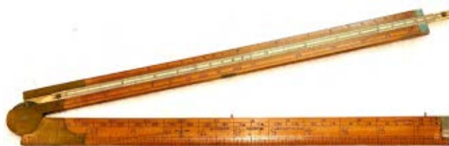
Fig. 6. A Typical Example of a Coggeshall, or Carpenter’s Rule, that Can Be Commonly Found in Many Tool and Slide Rule Collections Today
