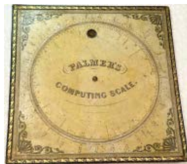
Fig. 14. The Palmer's Computing Scale, One of the First Slide Rules Manufactured in the US
