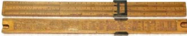
Fig. 12. An Early Example of a Mannheim Slide Rule by Tavernier-Gravet, 34 cm Length with Original Metal Cursor
