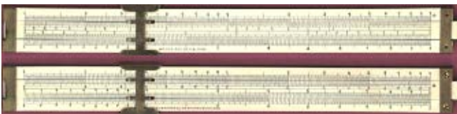
Fig. 13. Keuffel and Esser Cox Duplex, with Cursor Relating Calculations to Both Sides of the Rule
