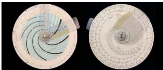
Fig. 9. The Culbertson Salinity slide rule (front and back), 1955, by Kahl Scientific, El Cajon, California.
