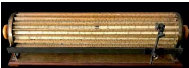
Fig. 4. Thacher's Calculating Instrument, 1907, by Keuffel and Esser, New York.
