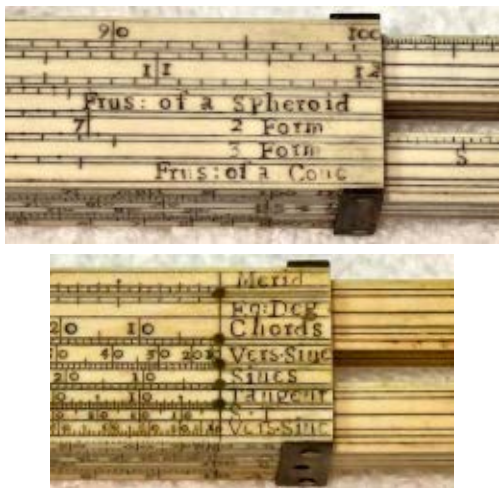
Fig. 19. An Early Ivory Slide Rule with both Excise and Gunter (Navigation) Scales
