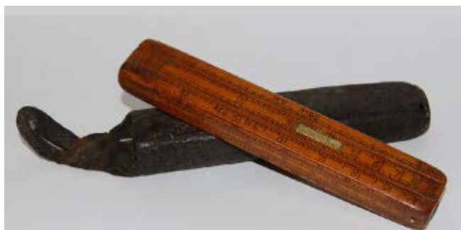
Fig. 1. An Everard-style Excise Tax Gauging Slide Rule, c. 1770, by Edward Roberts, London. Image courtesy of Nathen Zeldes.
