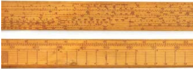
Fig. 2. Example of a Typical 19th Century 20-inch Gunter Scales with Gunter's Initial Scales and Numerous Others Added Later Proven Useful in Navigation
