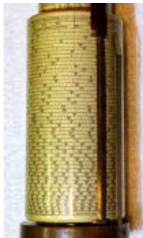
Fig. 16. Fuller Calculator One-Cycle Spiral Scale of 500 Inches in Length
